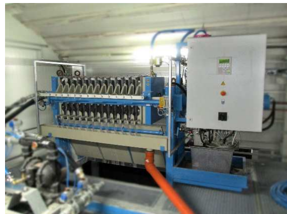
BIBKO®-Chamber filter press
