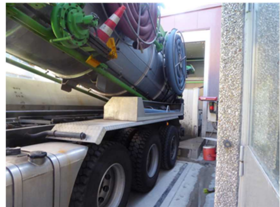
Emptying process suction/rinsing
